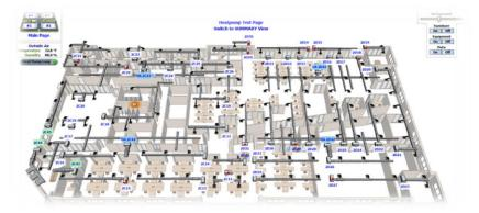
developed which shows all equipment, their locations, the ductwork, and
